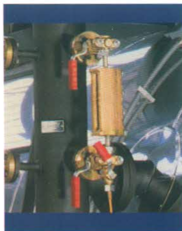
Side Water Level Indicator With Its Stop and Discharge Taps
